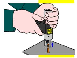
Visually inspect the weld. A good weld will result in an all round weld with a small visible witness of spatter surrounding the flange of the stud.
